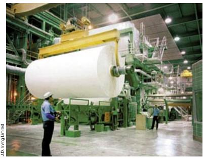
An overhead crane transfers a roll of paper to a winder at J.D. Irving tissue mill at Saint John, New Brunswick
