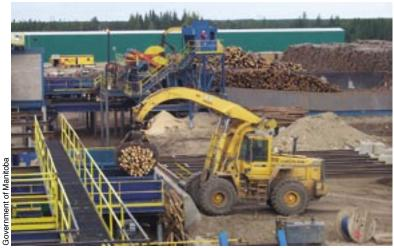
Sort yards like this one are used to separate softwood logs used in the manufacture of newsprint, kraft paper and lumber.
